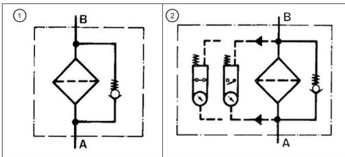
Bypass valve is integrated into the filter element.
